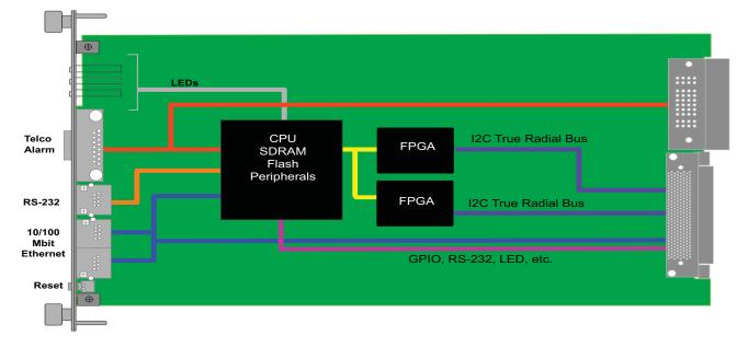
FIGURE 2. VT005 Functional Block Diagram
